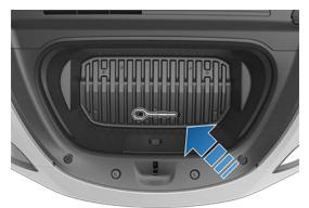
2. Release the rear tow eye cover by pressing firmly on its top right perimeter until it pivots inward, then gently pulling the raised section toward you.
