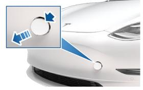
**3.** Fully insert the tow eye into the opening, then turn it **counter-clockwise** until securely fastened.
