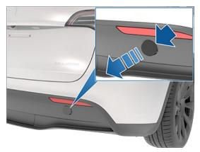
**3.** Fully insert the tow eye into the opening, then turn it **counter-clockwise** until securely fastened.
