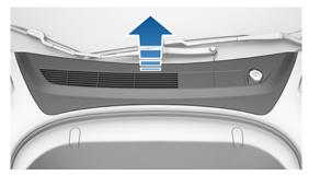
Remove the cabin intake trim panel by pulling it upwards to release the trim clips that hold it in place.
