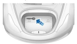
Release the tow eye cover by pressing firmly on the top right perimeter of the cover until it pivots inward, then gently pulling the raised section toward you.
